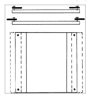
*Figure 1-4. Turning the steel rails increases spacing between them.*
