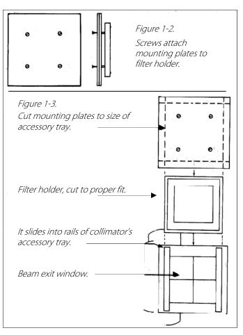
If the steel rails on the filter holder intrude into the x-ray field of view, unscrew the rails and turn them around (Figure 1-4). Since the screw holes in these rails are off center, turning the rails will set them <sup>3</sup>/<sub>4</sub>" further apart.
